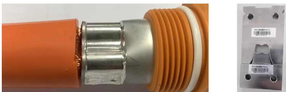
Figure 3.Example of double type B crimp
